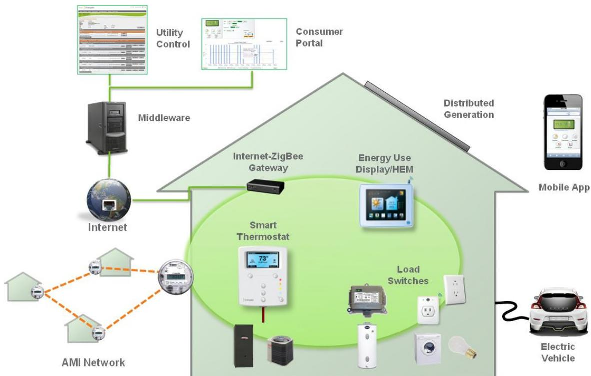
Figure 2: Shown here is a wireless ZigBee HAN served by both a broadband Internet gateway and an AMI network. Note the ability to control other loads, including the charging of electric vehicles, which will be supported in future versions of SEP.
