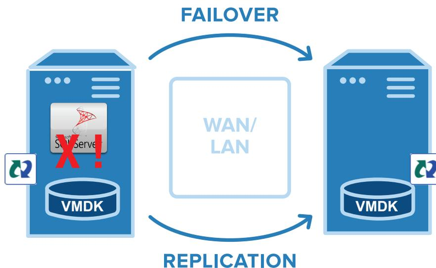
*In a SANless cluster, each VMDK can be attached to different VMs in an N-node cluster using each VM’s independent storage. The software provides LAN/WAN-optimized, real-time block-level replication in either a synchronous or asynchronous mode. In effect, it creates a RAID 1 mirror across the network. It automatically changes the direction of the data replication (source and target) as needed after failover and failback.*
