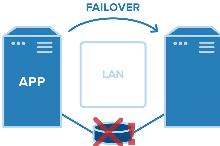
*In a traditional failover cluster, two or more physical servers (cluster nodes) are connected to a shared storage system. The application runs on one server, and in the event of a failure, clustering software such as Windows Server Failover Clustering (WSFC) moves the application to a standby node. Similar clustering is also possible with virtualized servers in a vSphere environment, but this requires a special configuration for the storage using Raw Device Mapping.*
